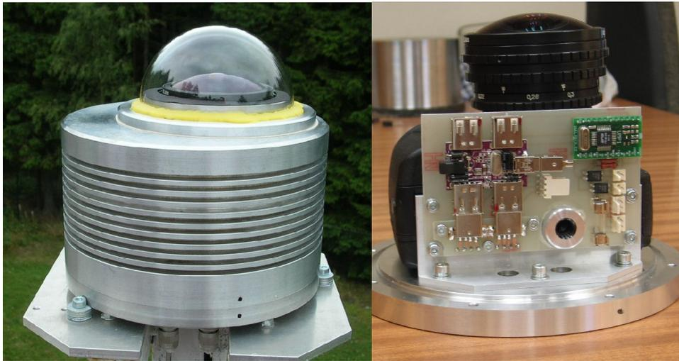
**Figure 1:** The assembled all-sky camera in observing conditions (left) and the camera with control electronic board (right)
