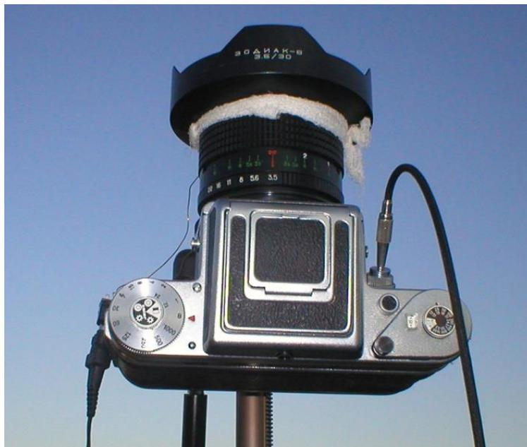
**Figure 4:** The Pentacon Six TL camera with the fish eye objective Zodiac. We expose on the 6 x 6 film, 400 ASA. The individual photos are exposed no longer than three hours.
