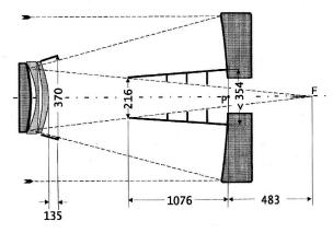
Figure 4: Optical layout of VNT
