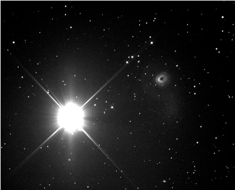
Figure 2: Example reflex image created by Paracorr coma corrector on 250 mm, f/4.8 Newtonian telescope. Reflex is center-symmetrical image of bright star Regulus, just above “Leo 1” dwarf galaxy.
